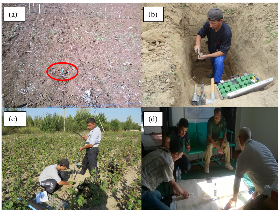
Photo 1: (a) TDR access tube for measuring soil-water content at different depths, (b) and (c) team collecting soil samples for soil characterization and determination of physical and chemical properties, and (d) team studying a historic HMZ map for selected Water User Association.
