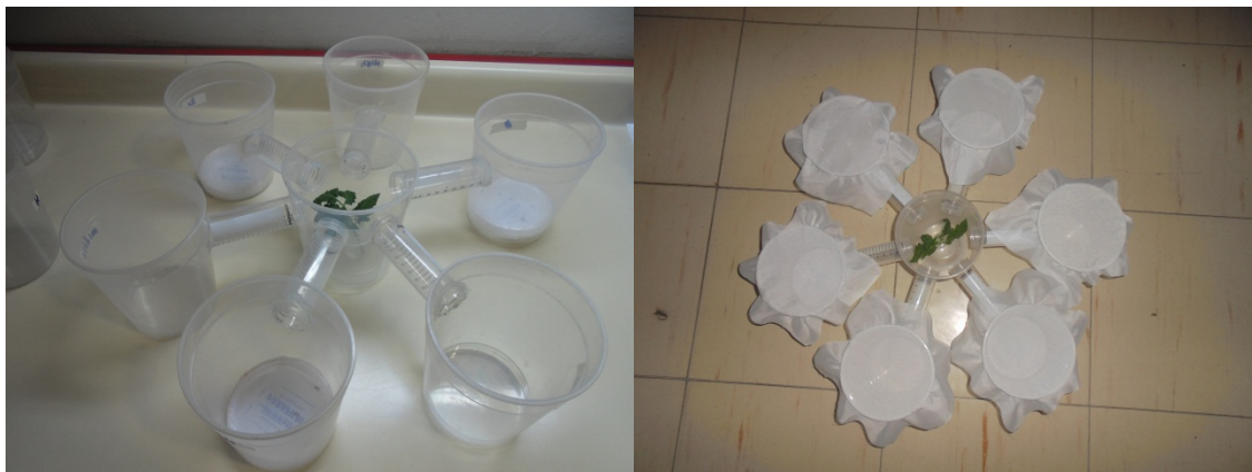
Figure 11. Six-armed olfactometer bioassay used to test preference of T. absoluta males between attract-and-kill formulations, differing in sex-pheromone concentrations and different numbers of virgine T. absoluta females
