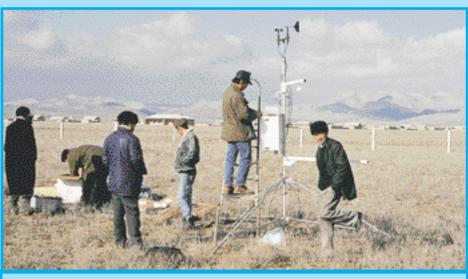
Installation of a carbon-dioxide Bowen Ratio Equipment at a site near Samarkand in Uzbekistan. The equipment will be used for carbon-dioxide flux monitoring.
