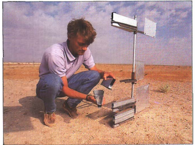
In a wind erosion project at Tel Hadya, the weight of dust collected in samplers was used to calculate the amount of material moved across a field.
