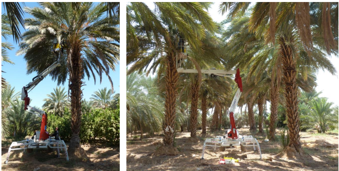
Figure 5.7 and 5.8. Placing for the two different methods: "360°" (left) and "180°+180°" (right).
