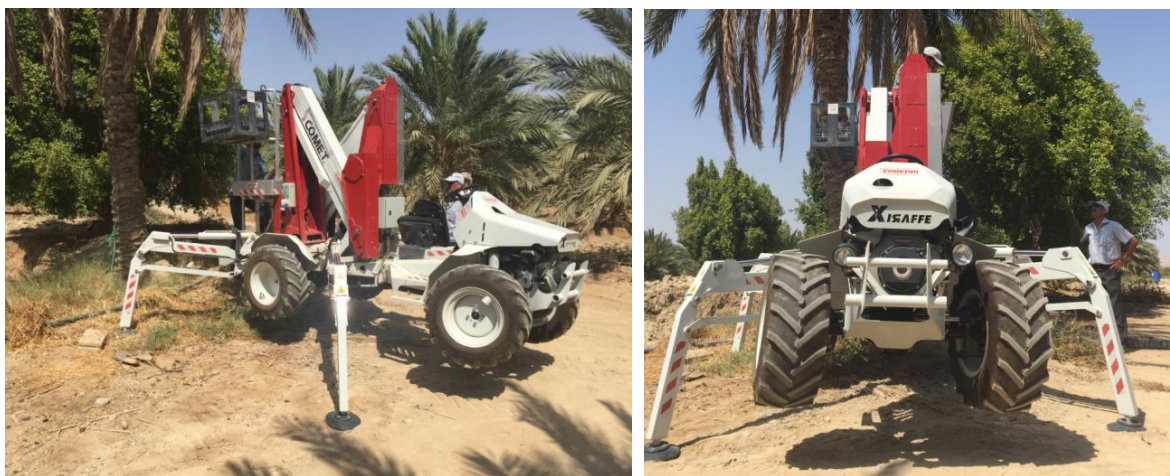
Figure 4.4 and 4.5. In the picture, Xiraffe vehicle after placing and ready for lifting operations.
