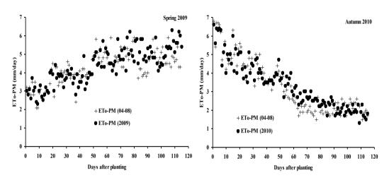
*Figure 2 - Day's reference evapotranspiration computed following the FAO-56 Penman-Monteith method. (ETo-PM) during the cropping seasons of potato for spring 2009 and autumn 2010 and period 2004-2008.*
