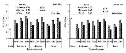
Figure 4 - Soil salinity (ECe, dS/m) under different irrigation treatments (FI100, DI-60 and DI30) for surface (SDI) and subsurface drip irrigation (SSDI) methods during the two cropping periods of potato. LSD (5%) indicates the least significant difference values at 5% level.
