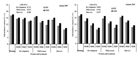
Figure 3 - Soil moisture content (%, v/v) under different irrigation treatments (FI100, DI-60 and DI30) for surface (SDI) and subsurface drip irrigation (SSDI) methods during the two cropping periods of potato. LSD (5%) indicates the least significant difference values at 5% level.
