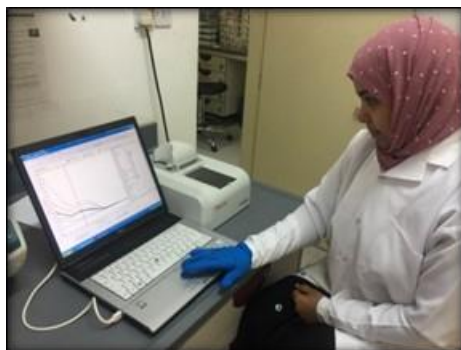
Fig. 2. Measuring the purity of the DNA using a device (Nanodrop).
