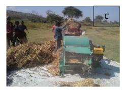
Figure 4. On-farm evaluation of engine driven common bean thresher at (a & b) at Shashemene and (c) at Ziway
