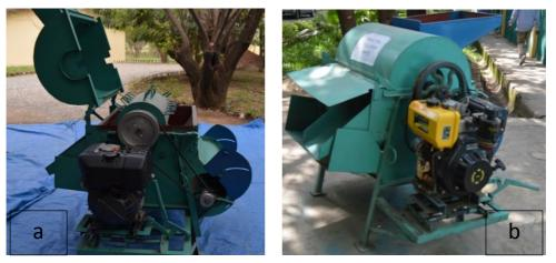
Figures 3 a) thresher after the pulley size is optimized b) the first pulley before its size is optimized for drum speed
