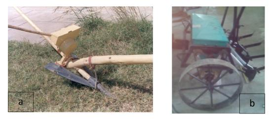
Figure 2. a) Erf and mofer attached row planter and b) recently developed Erf and mofer attached three row planter
