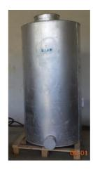
Figure 5. Metal silo storage prototype (1 ton capacity)
