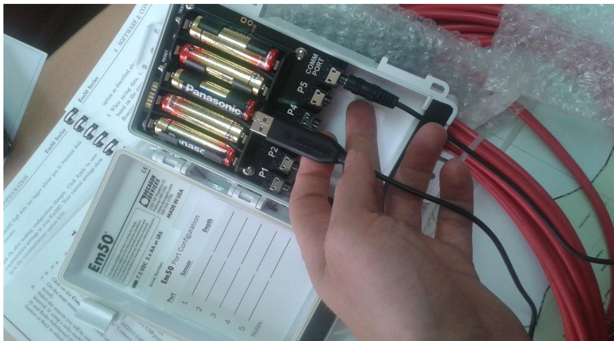
Fig. 3: Connecting the logger to the COMM PORT with the USB readout device. The USB port shall be connected to the computer
