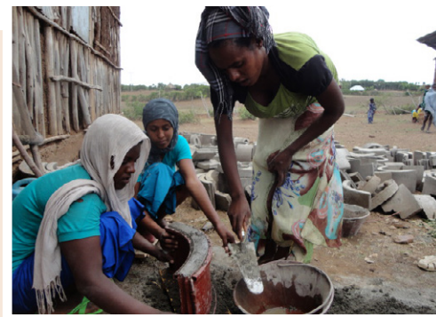
Young women engaged in mirt stove production using locally available cement, sand and water
