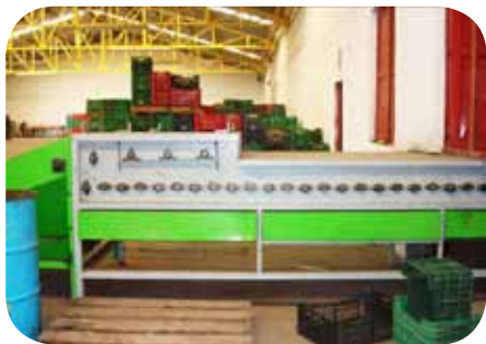
Figure 5. Cactus fruit cleaning machine in Mexico
