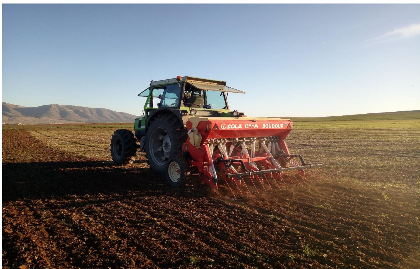
“Boudour” Zero-Till Seeder in the field (Credit: Nasreddine Louahdi, ITGC)
