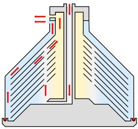
where the fat is directed to the cream outlet under the inner cover and the skimmed milk is directed to the outlet over the inner cover.
