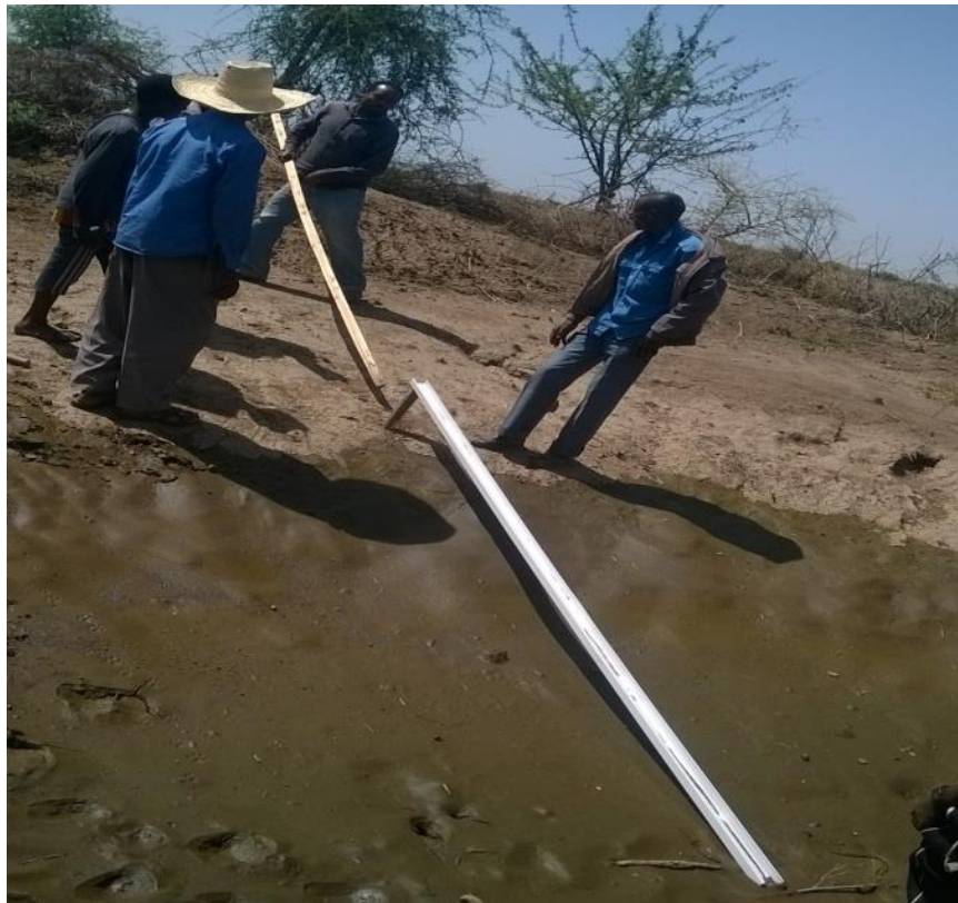
Figure 4: Installing a measuring system to record water levels in farm ponds.
