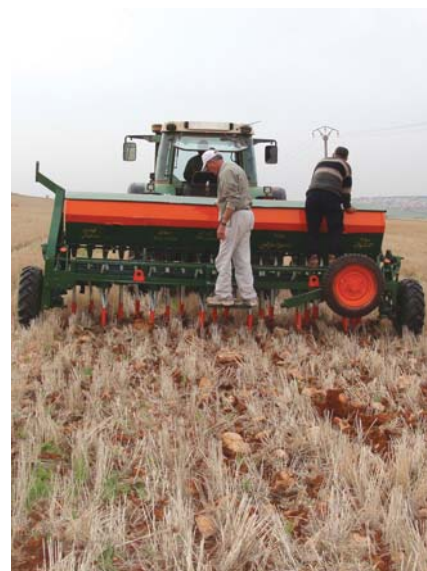
A low-cost zero-till seeder, developed by an Australia-ICARDA team in partnership with Syrian entrepreneurs
