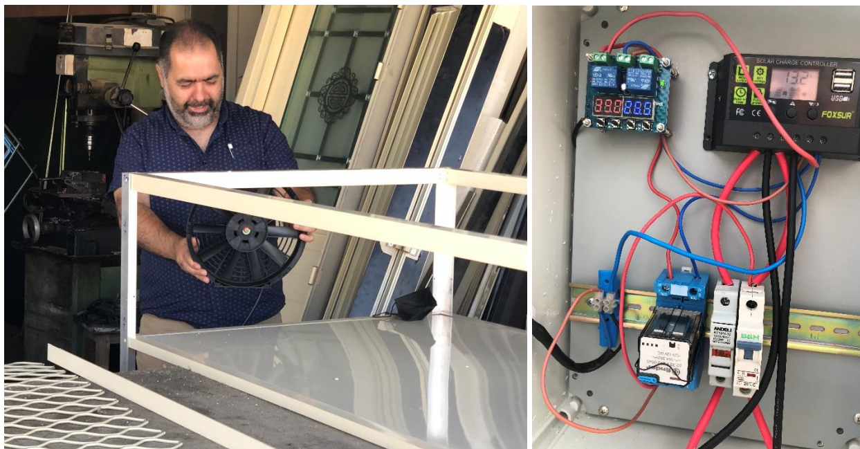
Picture 2. Solar dryer, UAE version. Left, frame at the manufacturing shop; Right, electronic board
