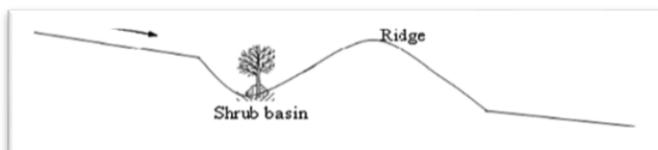
Figure 2 Typical layout of a micro catchment harvesting basin (Ali et al., 2010)
