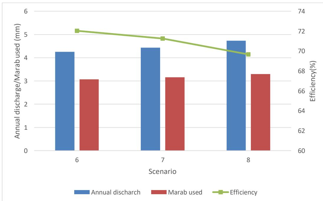
Figure 21 Annual discharge, used by the Marab and efficiency of discharge reaching the Marab with the 4, 6, 8 sub-watersheds with the highest discharge untreated
