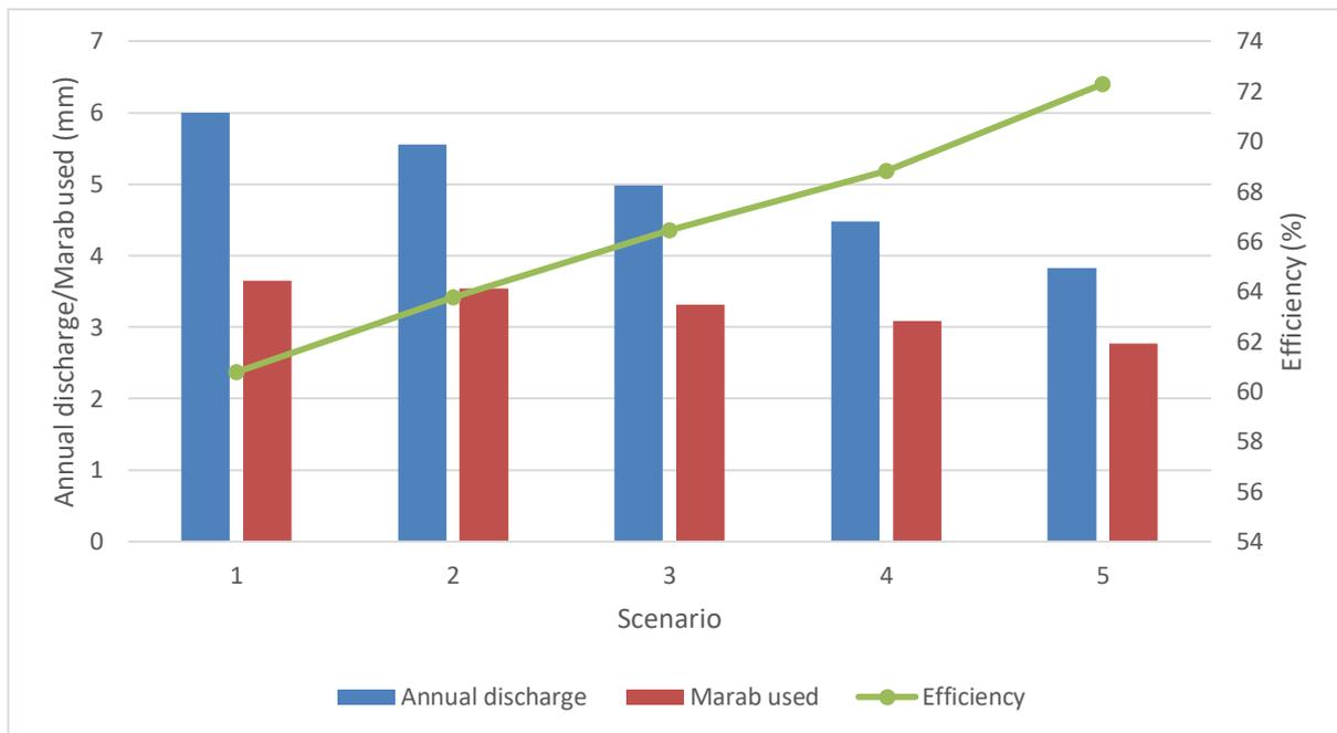
**Figure 17 Annual discharge, discharge used in the Marab and efficiency of water reaching the Marab for 5 scenarios with different numbers of Vallerani structures implemented**
