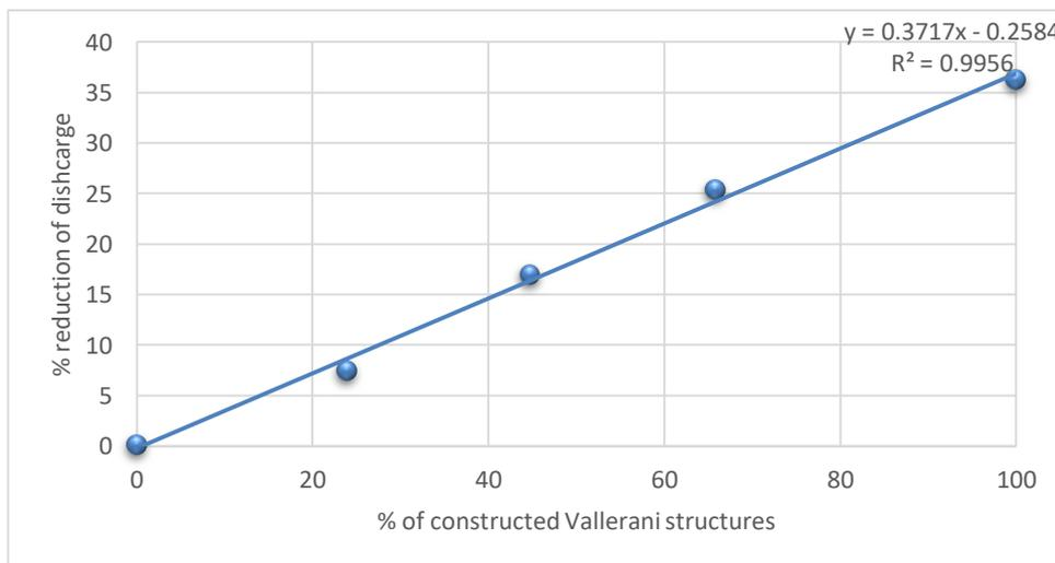
Figure 20 Reduction of discharge reaching the Marab due to the implemented Vallerani structures in the watershed
