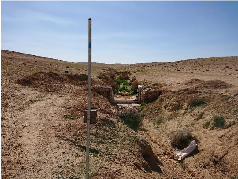
Figure 9 Discharge measurement setup for the untreated sub-watershed
