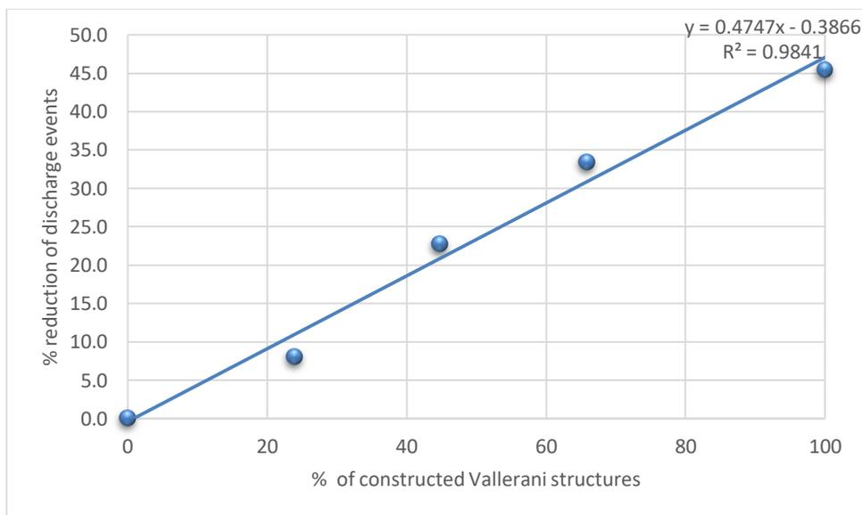
Figure 16 Reduction of discharge events in the Marab due to implementation of Vallerani structures in the watershed
