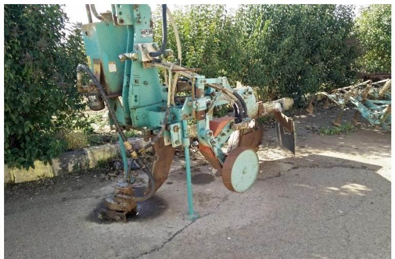
Figure 3 Plow used to make Vallerani structures
