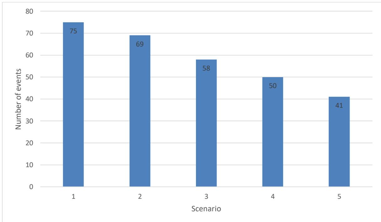
Figure 15 Number of discharge events in the Marab modelled over a 30-year modelling period for 5 scenarios with different numbers of Vallerani structures implemented in the watershed
