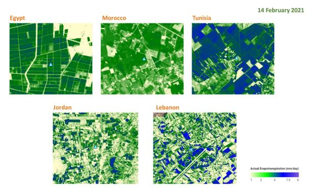
Figure 50: SEBAL GEE based actual evapotranspiration of study locations during peak vegetative stage of different crops during 2021. The triangle (cyan colored) depicts the field ETa observation site
