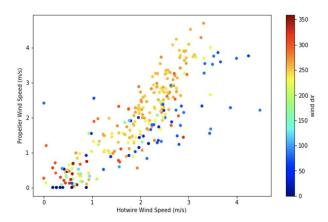
**Figure 63:** Validation of the wind speed comparing the hot wire with the wind speed measured at the weather station. The colors represent the wind direction. Note how the estimates of the wind speed decline with wind directions are in the range 0-100 degrees.
