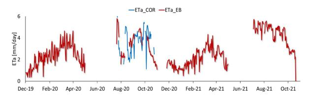
Figure 6a ETa measured at the Sakha Site, Egypt, by the on-site approach of Energy Balance (ETa\_EB).
