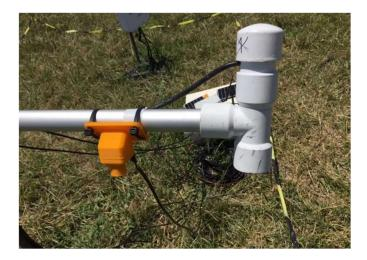
**Figure 65:** Infrared thermometer (Melexis MLX90614) in an orange 3D printed housing installed next to an IRTS-P Apogee sensor.
