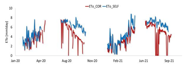
Figure 13 ETo measured at the Dyar Ala Site, Jordan by CORDOVA-ET Station (ETo\_COR) and inhouse approach (ETo\_SELF).
