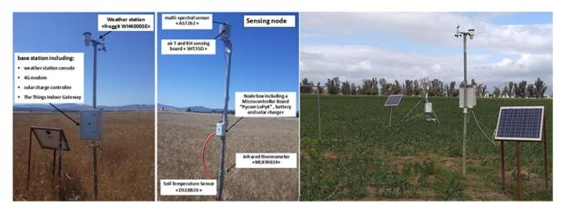
Figure 36 The location and the assembly details of the CORDOVA-ET Station at the El Khoudia site, Tunisia.
