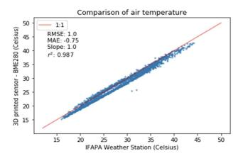
**Figure 57:** Validation of air temperature sensor, comparing the CORDOVA sensor in the 3D printed radiation shield and the standard sensor in the IFAPA weather station.
