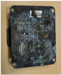
**Figure 67**: Water ingression in a IP67 box resulted in damaged electronics and total failure. Despite the use of outdoor rated gland nuts, this box was not suited with a vent valve that facilitated water sipping through the glen nuts with the changes of pressure.
