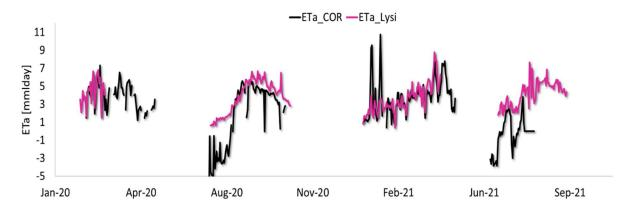
Figure 14a ETa determined at the Dyar Ala Site, Jordan, by CORDOVA-ET Station (ETa\_COR) and in-house approach, which was a weighing lysimeter (EaT\_Lysi).
