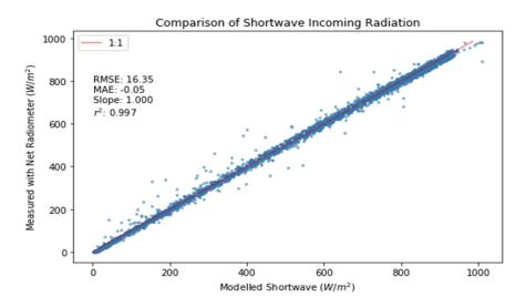
**Figure 61:** Comparison of solar radiation for the multispectral sensor and the pyranometer from the net radiometer. The calibrated values from the multispectral sensor are obtained using multivariate regression that combines all the spectral bands and sensor temperature.
