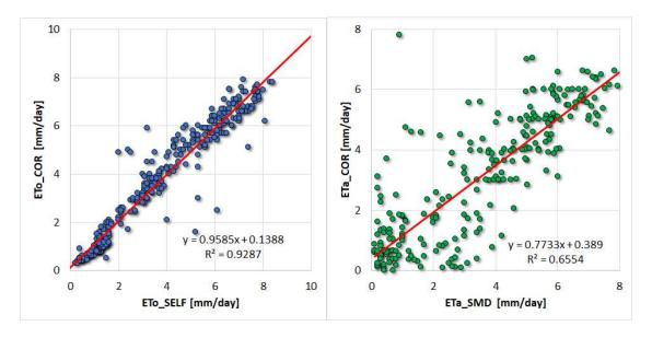
Figure 21b Statistical comparisons between the different estimates of ETo and ETa, respectively. A linear regression ( $y=6_1x+6_0$ ) was evaluated.  $R^2$  explains the percentage of the variance in the dependent variable that the independent variables explain collectively.
