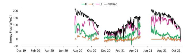
Figure 7 Components of the Surface Energy Fluxes (H- Sensible Heat Flux, LE Latent Heat Flux, G- Ground Heat Flux along with Net Radiation Flux) at the Sakha Site, Egypt.
