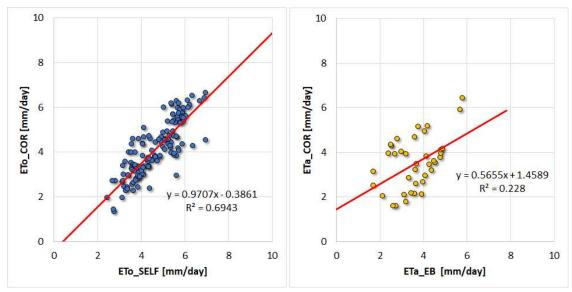
Figure 6b Statistical comparisons between the different estimates of ETo and ETa, respectively. A linear regression ( $y=\theta_1x+\theta_0$ ) was evaluated.  $R^2$  explains the percentage of the variance in the dependent variable that the independent variables explain collectively.
