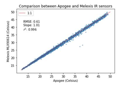
Figure 66: Validation of the infrared temperature of the MLX90614 sensor compared with the Apogee IRTS-P sensor.
