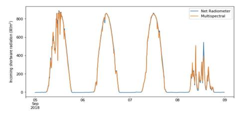
Figure 60: Evolution of solar radiation measured with the net radiometer and modelled from the multispectral sensor.
