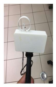
**Figure 62:** Test prototype for the CORDOVA wind speed sensor. A ring protective ring was added to protect the sensor from birds and any accidental damage. The box contains the electronics for powering and sensing.
