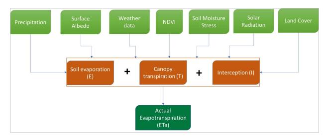
Figure 47: Brief indicative methodology for ET estimation using ET-Look model, ETa data available on Water Productivity Open-access Portal (WaPOR)
