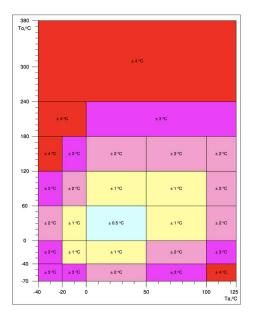
**Figure 64:** Accuracy of the CORDOVA IRT sensor depending on the object and ambient temperature. For the normal range of operation in agricultural applications the accuracy is 0.5°C.
