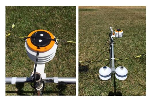
**Figure 59:** (a) Top view of the spectral sensor in the enclosure with the optic diffuser. In this test model, two sensors can be installed for simultaneous observation or for including visible and near infrared versions of the spectral sensor. (b) pyranometer and net radiometer (NR-01, Hukseflux, The Netherlands) used for the calibration.
