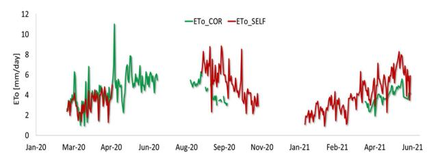
Figure 28 ETo measured at the Berrechid Site, Morocco, by CORDOVA-ET Station and inhouse approach.
