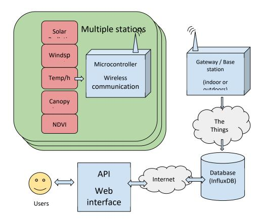
Figure 55. Overview of the CORDOVA-ET system. Multiple stations with the sensors and wireless communication (LoRaWAN) are deployed in the field. A gateway/base station receives the information from the stations and forwards the information to the Internet. The data is stored in a database and it is exposed to the users through a web interface and a programming API accessible with R and Python.
