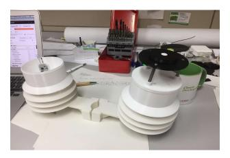
**Figure 56.** 3D printed radiation shields and sensor boxes containing the air temperature, humidity and barometer, hot wire anemometer and solar radiation sensor (on the right).
