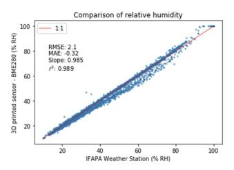
**Figure 58.** Validation of air humidity sensor, comparing the CORDOVA sensor in the 3D printed radiation shield and the standard sensor in the IFAPA weather station.
