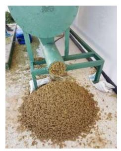
Figure 5: Pellets produced from local materiel (Udo Rudiger/ICARDA)
