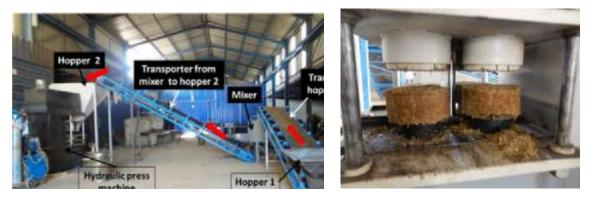
Figure 2 : Feed block manufacturing unit and produced feed blocks (Ali Nefzaoui/ICARDA)
