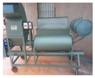
Figure 4: Locally manufactured pellet machine (Udo Rudiger/ICARDA)
