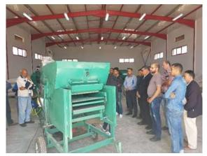
Figure 10: Mobile seed cleaning and treatment unit (Zied Idoudi/ICARDA)
