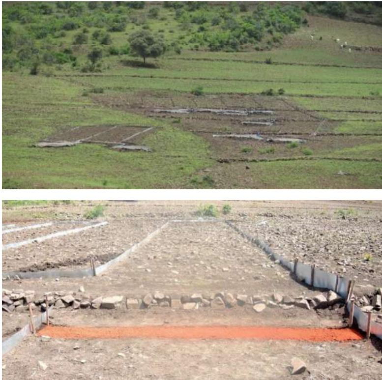
Figure 4. Overview of the erosion site (top image), and the tracer experiment (colored tracer stripe (iron oxides)) carried out at the cumulative hill slope plot (bottom image).
