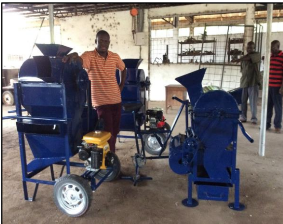
Gabriel Abdulai and the original three SIL soybean threshers for smallholder farmers. This design was dropped after field testing with farmers in Ghana
