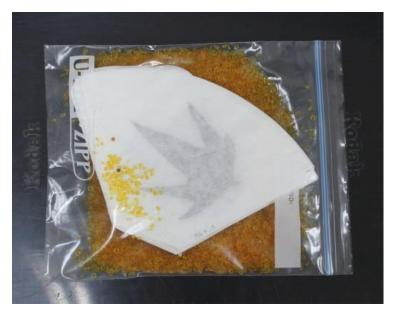
Figure 2. Orange silica gel with the leave sample inside a coffee filter into Ziplock bags
