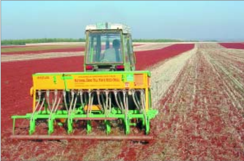
Direct-drilling equipment from India, originally designed for rice, is being adapted for use in wheat and intercropping systems.
