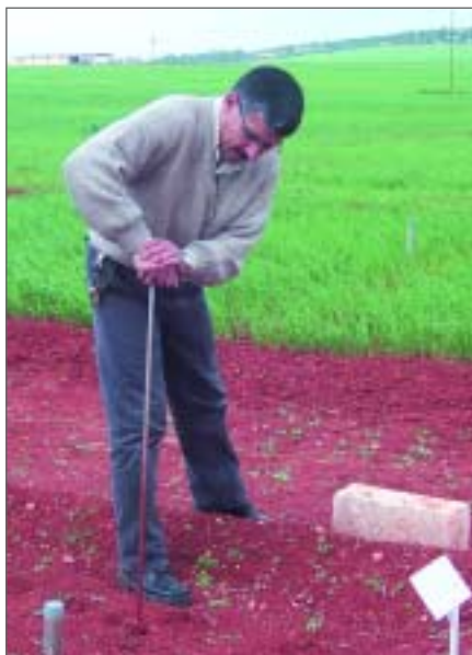
The Water Wand is a low-cost, easy-to-use probe for estimating soil moisture and compaction.
