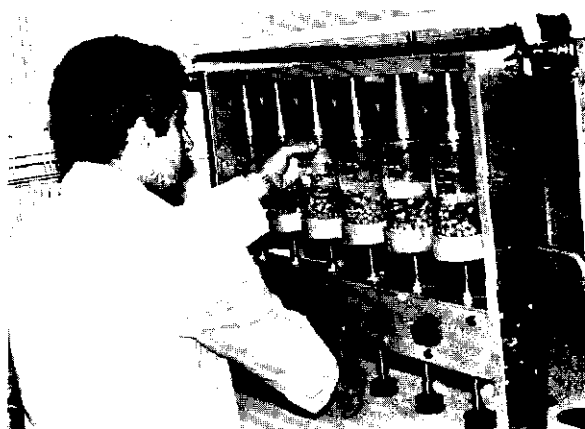
The cooking quality of kabuli chickpeas is being evaluated using the Labconco Crude Fibre Digestion System.
