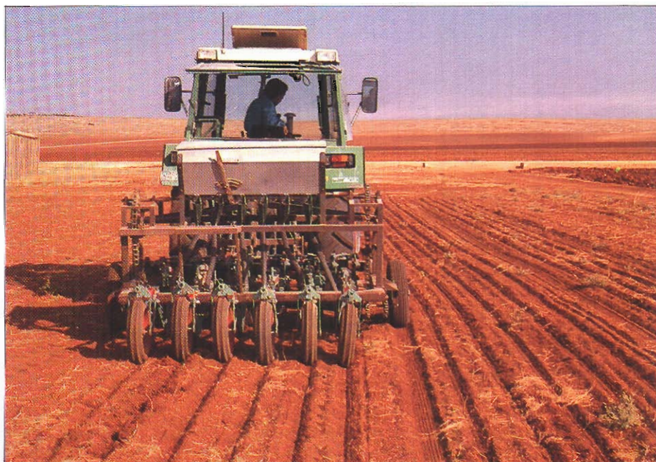
A zero-till planter has been assembled at ICARDA using imported commercial units and a locally built seed box.
