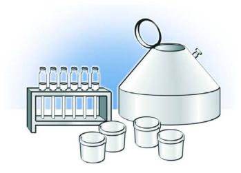
Butyrometer is used to measure fat content of milk
