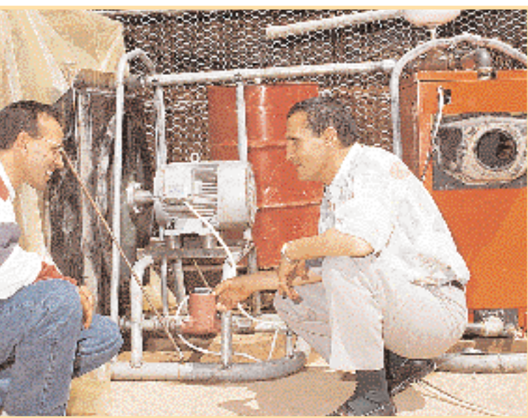
Dr Hassan Ouabbou (left) and Dr Mohamed Iskandar with the sirocco simulator. The boiler, at right, was a spare; a more normal heat source would be an ordinary domestic diesel-burning water-heater, of a type which is in common use all over the Maghreb and Mashreq regions.
