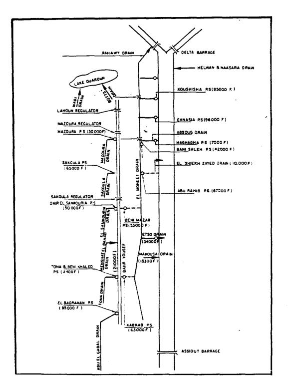
Fig. 6. Drainage system from Assiut to the Delta.
