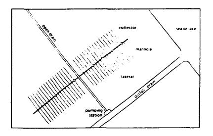
Fig. 3. Covered drainage system used in Egypt.
