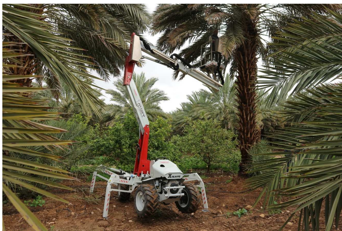
Fig. 19: Light off-road platform for easy access to higher palms in traditional palm groves (Photo credit: Garbati Pegna)
