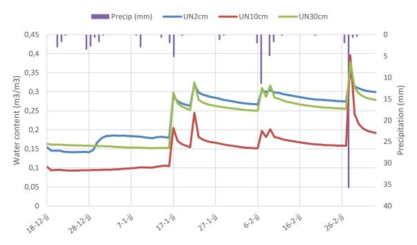
Figure 12 Soil moisture measurements obtained from Decagon 5TE sensors at depths of 2 cm, 10 cm and 30 cm underneath the furrow of a Vallerani RWH structure from the 18<sup>th</sup> of December 2018 till the 6<sup>th</sup> of March 2019. Measured precipitation values for the same period on the secondary axis.
