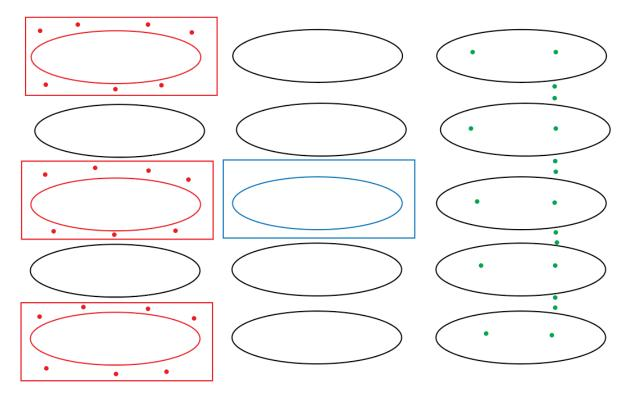
Figure 5 Schematic overview of the hillslope on which the experiments took place. In red the Vallerani RWH structures a long which photogrammetry was performed. Blue outline is the structure around which the Decagon 5TE sensors were installed (Figure 9 for detailed placement). Green dots are the TRIME-PICO sensors.
