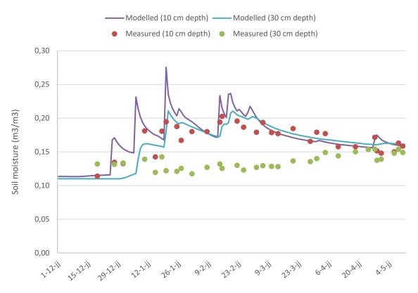
Figure 18 Modelled and measured soil moisture values downstream of the Vallerani RWH structure at depths of 10cm and 30cm for a period from the 1st of December 2017 till the 5th of May 2018. Measured soil moisture values obtained using TRIME-PICO sensors.
