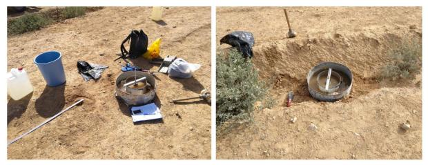
Figure 6 Test site set up of the double-ring infiltrometer. Inside the furrow (right) and on the hillslope (left).
