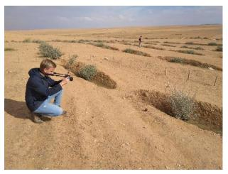
Figure 8 Photogrammetry being performed in the field.
