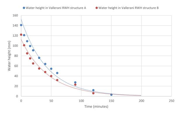
Figure 11 Water height over time in two Vallerani RWH structures during the fill experiments. Structure A is the Vallerani RWH structure containing the Decagon 5TE sensors. Structure B is the second Vallerani RWH structure that was filled.
