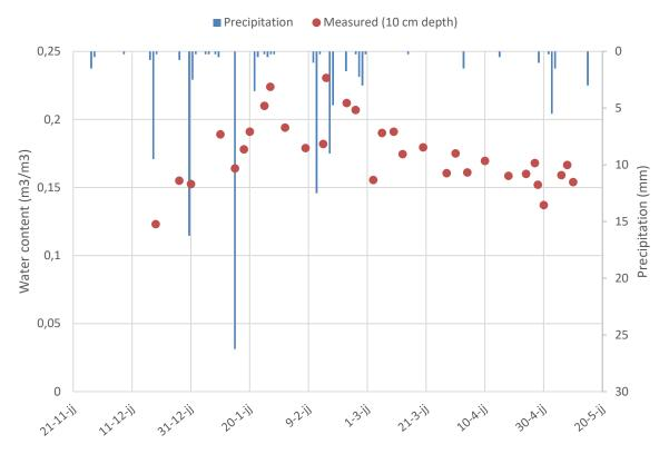
Figure 15 Soil moisture measurements values obtained from the TRIME-PICO sensor at a depth of 10 cm upstream of the furrow of a Vallerani RWH structure from the 19<sup>th</sup> of December 2017 till the 10<sup>th</sup> of May 2018. Measured precipitation values from the 21<sup>st</sup> of November 2017 till the 20<sup>th</sup> of May 2018 on the secondary axis.
