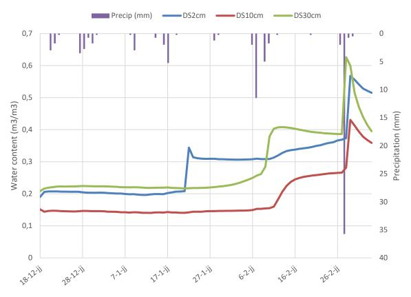
Figure 13 Soil moisture measurements obtained from Decagon 5TE sensors at depths of 2 cm, 10 cm and 30 cm downstream of the furrow of a Vallerani RWH structure from the 18<sup>th</sup> of December 2018 till the 6<sup>th</sup> of March 2019. Measured precipitation values for the same period on the secondary axis.
