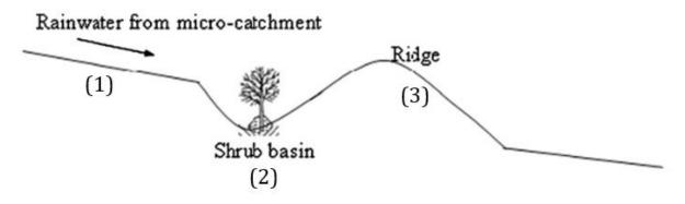
Figure 1 A schematic overview of a micro rainwater harvesting structure. (Taken from Ali et al., 2010)
