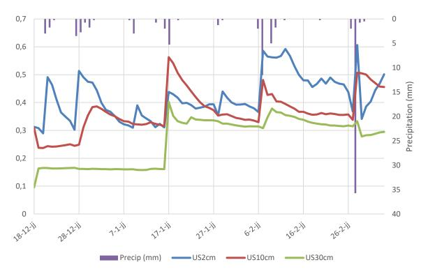
Figure 14 Soil moisture measurements obtained from Decagon 5TE sensors at depths of 2 cm, 10 cm and 30 cm upstream of the furrow of a Vallerani RWH structure. From the 18<sup>th</sup> of December 2018 till the 6<sup>th</sup> of March 2019. Measured precipitation values for the same period on the secondary axis.
