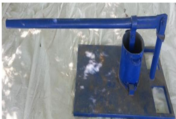
Figure 57. Manual feed block machine in Yemen
