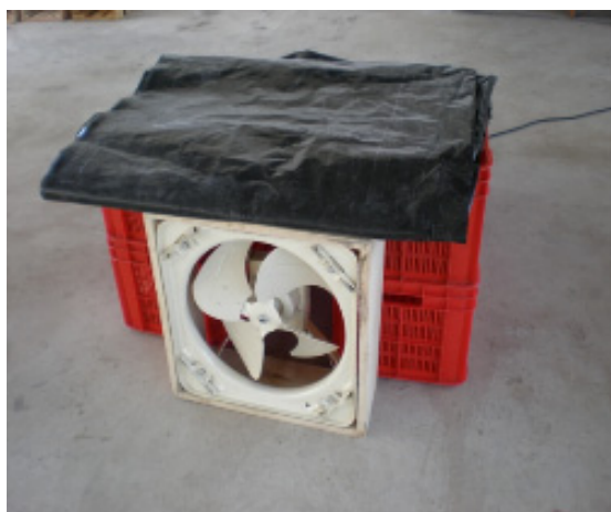
Figure 50. Photograph of a fan and its flexible cover used for pre-cooling vegetables in a cold room
