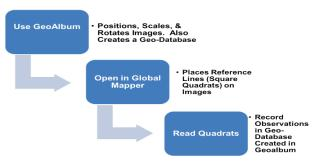
Figure 5. The office process involves positioning, rotating, and scaling images and saving them as geo-registered bitmaps.
