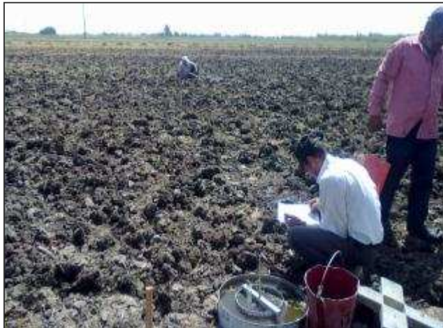
Infiltration rate using double ring cylinder infiltrometer
