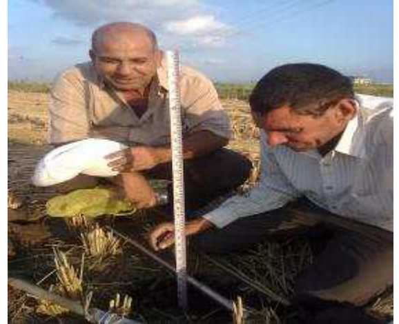
Hydraulic conductivity (K) using the auger-hole method
