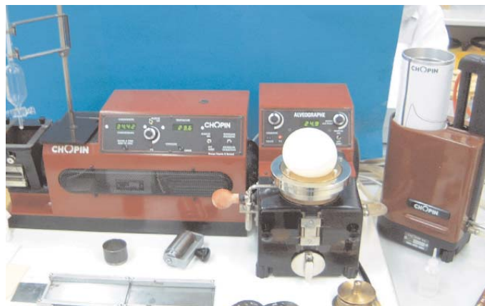
Alveograph for evaluating gluten extensibility, an important quality for making bread.
