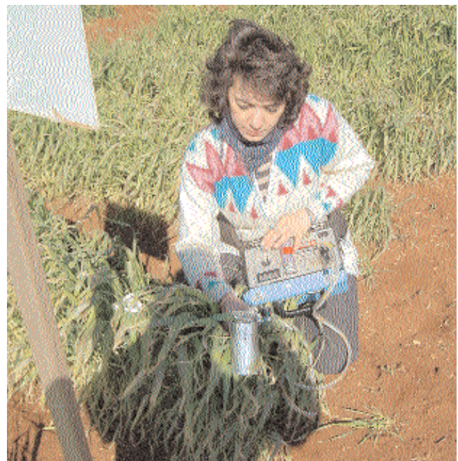
Measuring water-use efficiency (leaf temperature, quantum yield, stomata resistance/conductance and transpiration) with a porometer in a durum field at Tel Hadya.
