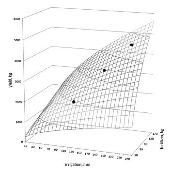
**Fig. 3.** Illustration of CropSyst yield simulation for different irrigation and fertilizer use in the example of wheat.
