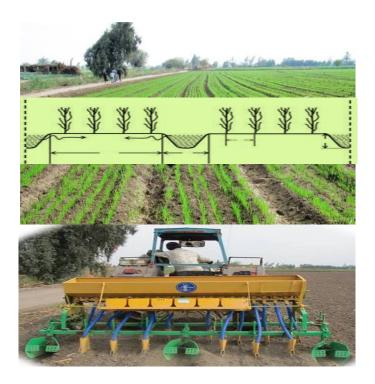
Figure 6. Mechanized raised bed wheat plantation in the Delta of Egypt. (ICARDA, 2013)
