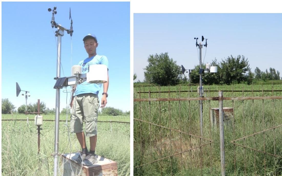
Figure 8. Establishment of automatic weather station at Khorezm Station of Cotton Breeding, Seed Production and Agro-technologies
