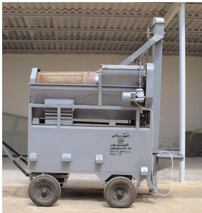
A mobile seed-processing machine developed in Syria for farmers in Afghanistan and other countries.
