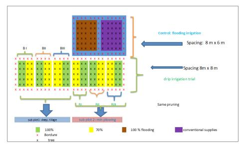
Fig. 1. Experimental design at Tessaout research stations near Marrakech, Morocco.
