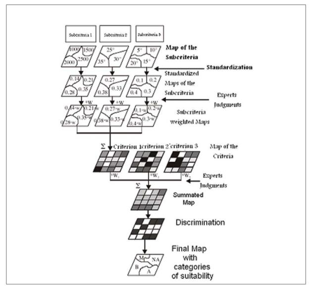
Figure 3.4. Aggregation sequence of classes and weights for the hierarchies defined in the application of the spatial AHP to define areas of different suitability in the upper catchments. (Adapted from Bustillos-Herrera *et al.*, 2007). Chapter 4.
