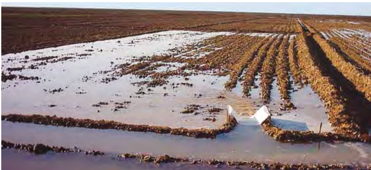
Fig. 2.7. Measurement of flow to the irrigation border
