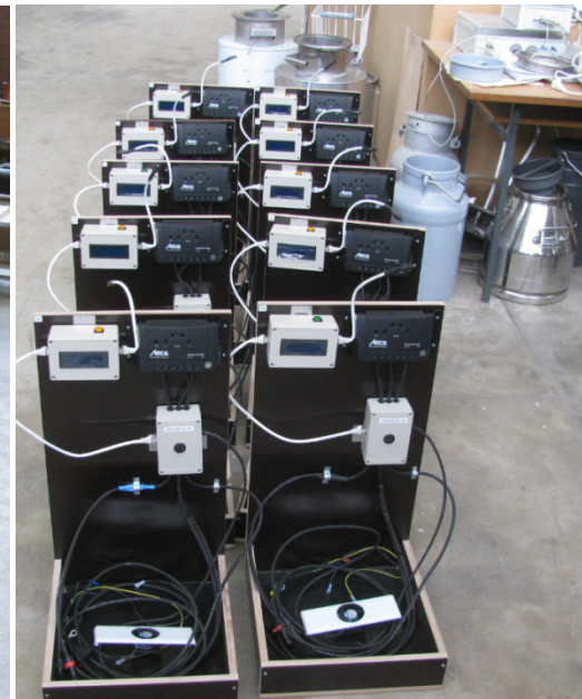
Control panels with charge controller, data logging and fan
