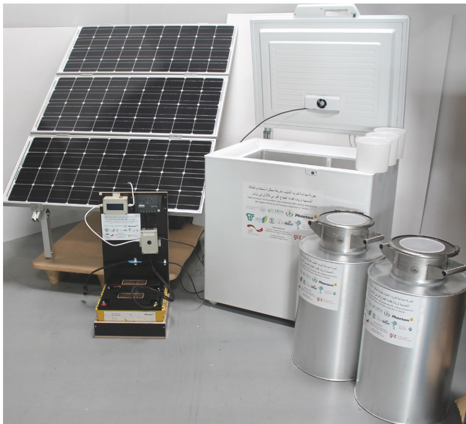
One of the 10 systems shipped to Sidi Bouzid (PV Panels, 2 Batteries, Control panel, Solar freezer, 25 ice-tins, 2 Milk cans)
