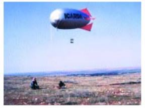
In a cooperative project between ICARDA and Japan, a video-monitoring camera takes photographs from a balloon 200 meters above ground in Syria. Vegetation maps developed from the photogrpahs are verified against LANDSAT satellite images to determine species distribution and the changes caused by overgrazing.
