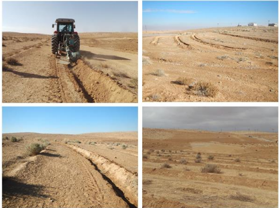
Figure 4. The minimum tools for an arid rangeland restoration project: using a tractor with two-furrow plow to make a Vallerani micro water-harvesting catchment
