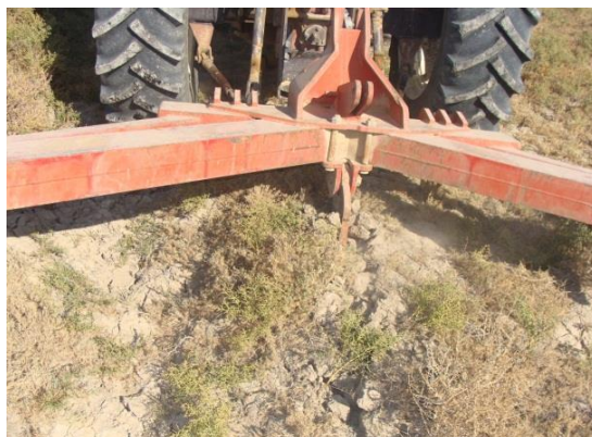
Fig. 8. Use of rotor to breakdown hardpan in deep plowing at Dujaila
