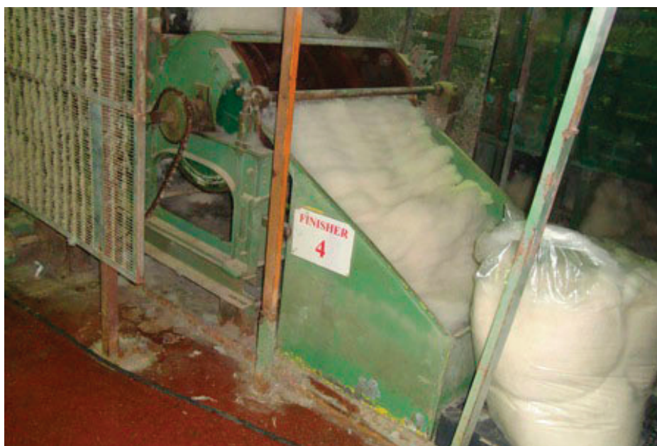
Figure 73. Complimentary dehairing; Sefit Pajan processing mill in Semnan province.
