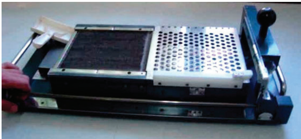
Figure 77. Staple length lining apparatus; Sefit Pajan processing mill, Semnan province.
