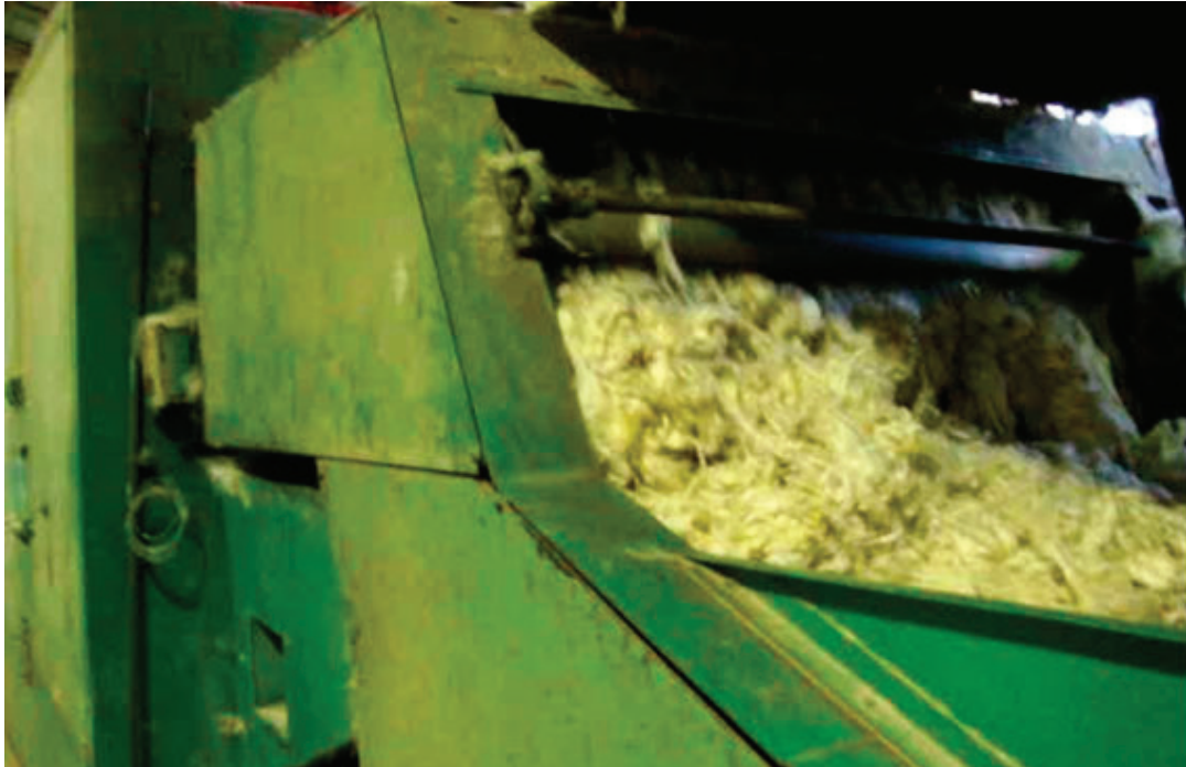
Figure 62. Air flow dryer; Sefit Pajan processing mill in Semnan province.
