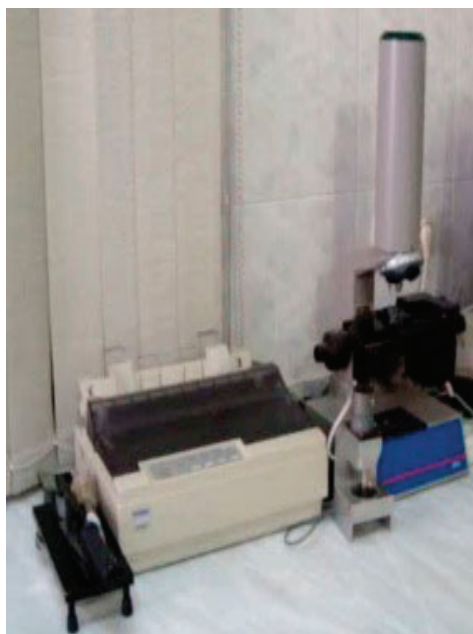
Figure 76. Fiber diameter and cashmere yield measurement apparatus. Sefit Pajan processing mill, Semnan province.
