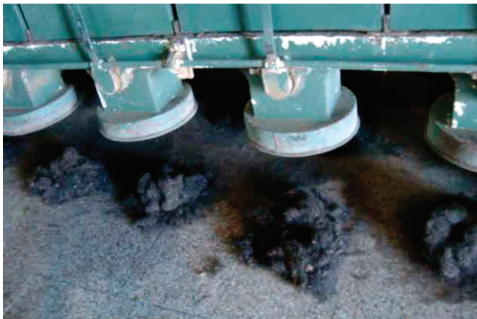
Figure 68. Guard hair and cashmere waste is discarded from the exit valves beneath garneting machine. Mashad processing mill in Khorasan Razavi province.
