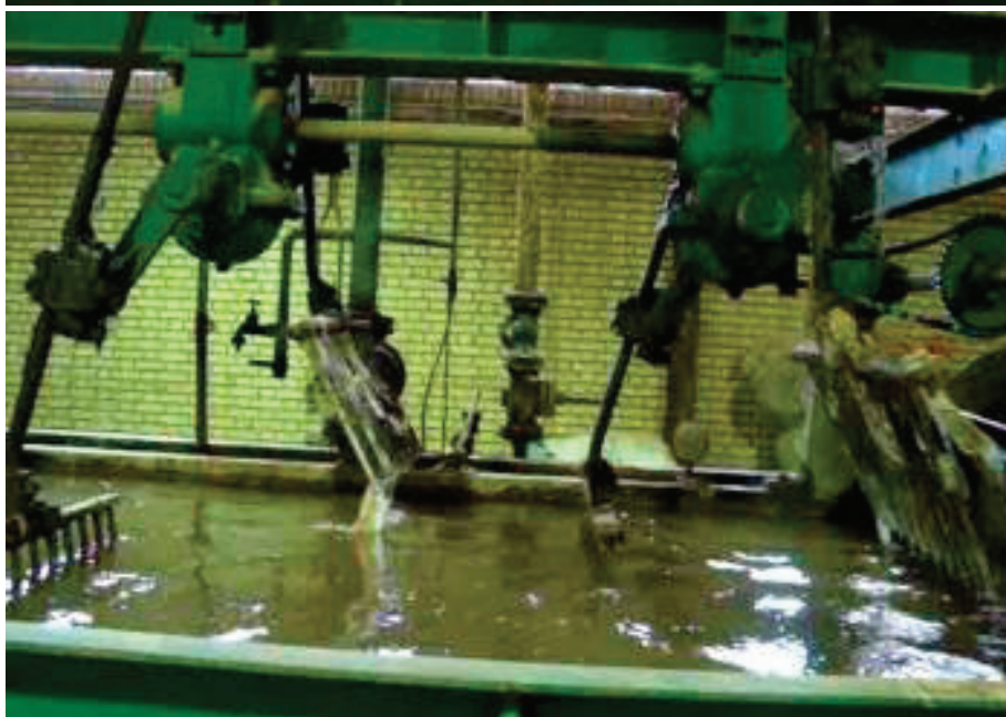
Figures 60 and 61. Cashmere scouring machine: first and second bowls propulsion and extraction by Harrows. Sefit Pajan processing mill in Semnan province.
