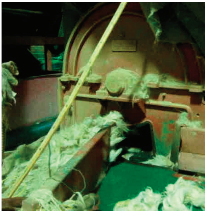
Figure 59. Double-cylinder cashmere opener; Sefit Pajan processing mill in Semnan province.
