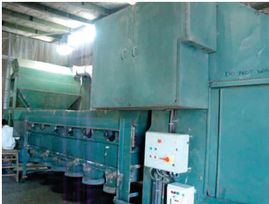
Figure 67. Garneting machine, short cashmere fiber is manually fed into the machine; Mashad processing mill in Khorasan Razavi province.
