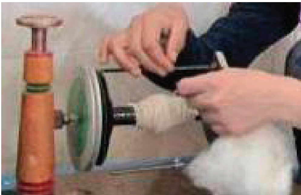
Figure 26. Small electrical machine for making yarn.
