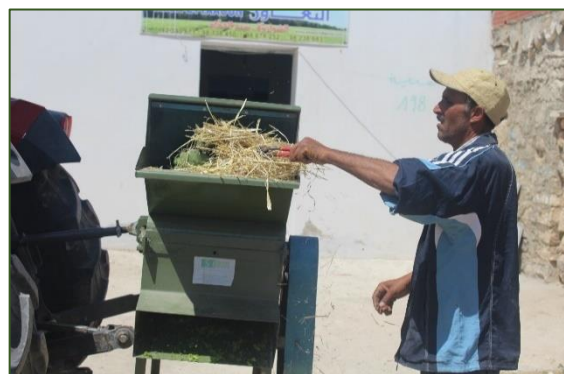
Small-scale feed grinder to improve the quality of roughage feed (Tunisia)
