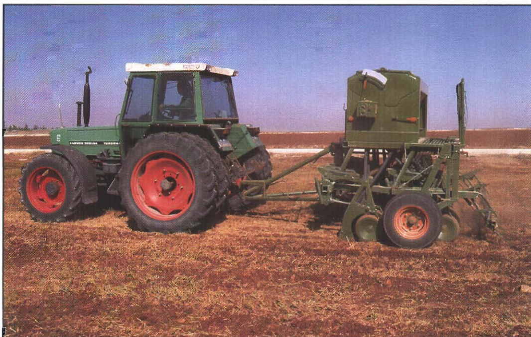
0-till planter and fertilizer bander at work at Tel Hadya.
