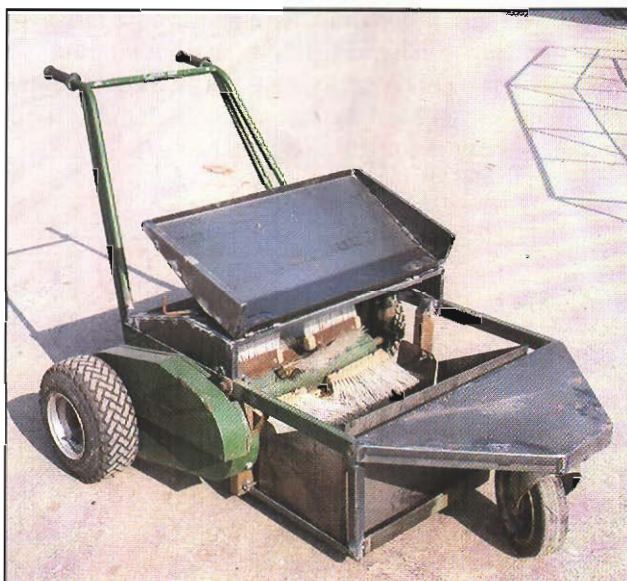
Pasture legume pod collector developed by ICARDA.
