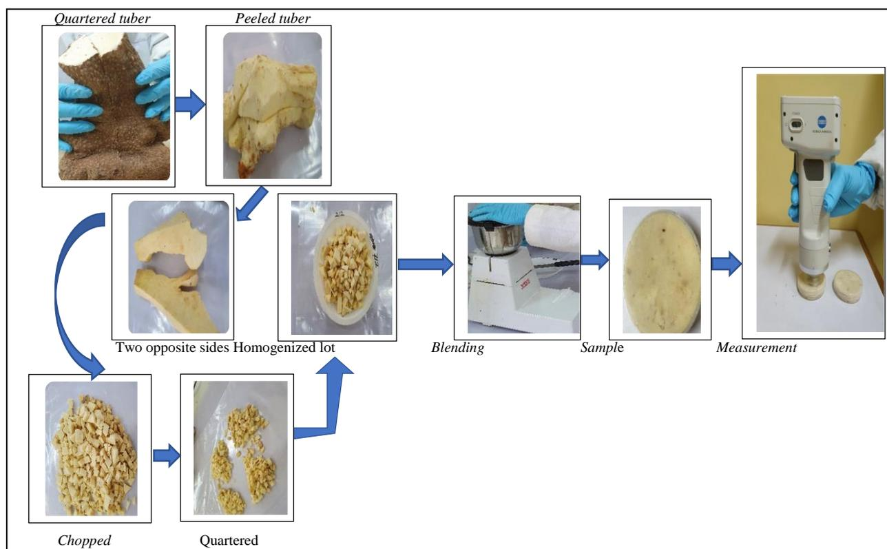
Figure 1: Workflow of color measurements using a Chromameter
