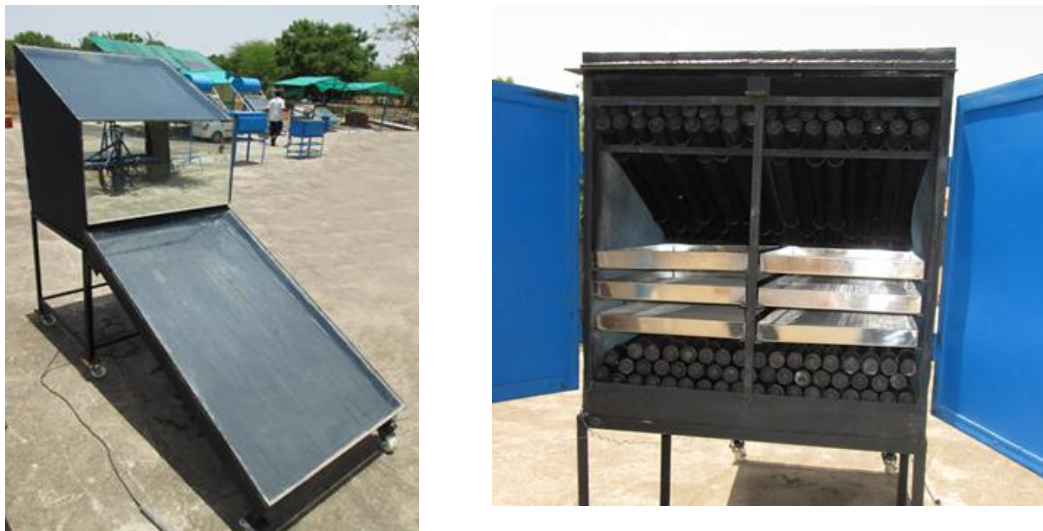
Figure 9. Solar dryer with PCM thermal energy storage (Jain and Tewari, 2015)
