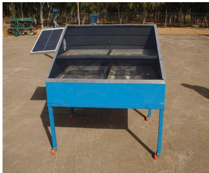
Figure 3. Photovoltaic/thermal (PV/T) hybrid solar dryer (Poonia et al. , 2018).
